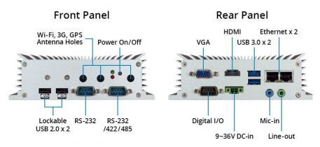
The Automation Conductor is a fanless PC system utilizing, which includes USB 3.0, USB 2.0, Low-powered DDR3 and dual Ethernet ports. The system is ideal for industrial control systems, SCADA. deviceWise® ready; and Verizon certified.
